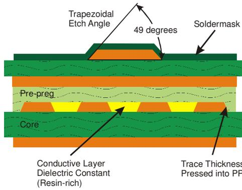
Figure 4. Allegro cross-section features
