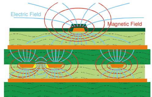
Figure 7. Field lines associated with single-ended and differential traces.
