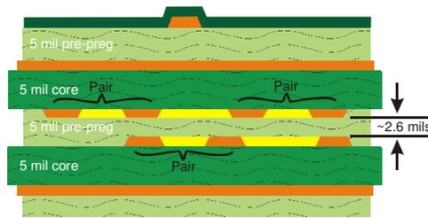
Figure 9. Cross section for the brave! Crosstalk simulation is the only safe way forward.
