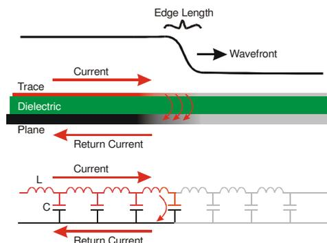
Figure 2. Transmission line propagation on PCB microstrip and equivalent ideal model
