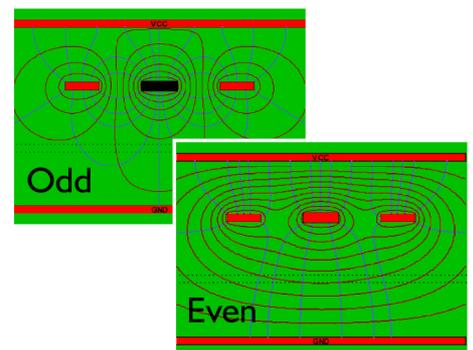
Figure 8. Odd and even mode field lines
