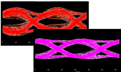
Fig1. Altera HSSIO DML simulations showing effect of varying link differential impedance.
