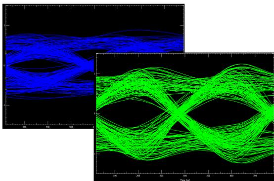
Fig3. Xilinx RocketIO™ HSPICE® simulation. The vertical opening is increased 3x by PCB design alone.
