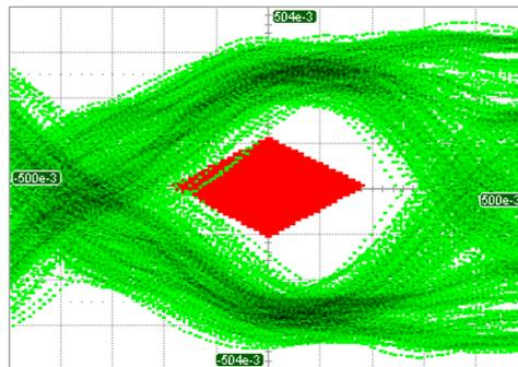
Fig2. Compliance eye showing mask violations - with so little room for error we must design every section of MGHZ interconnect with care.
