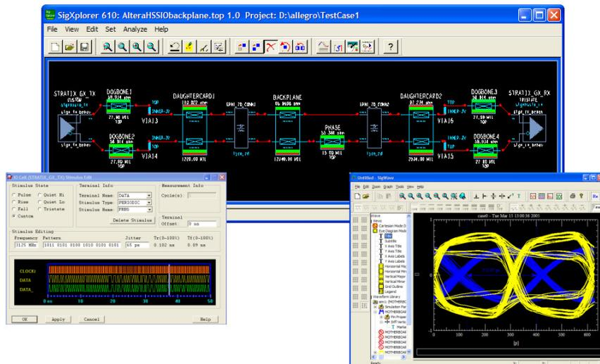
Fig4. "Allegro® PCB SI™ - proactively addresses issues typical of 3.125-Gbps links."
